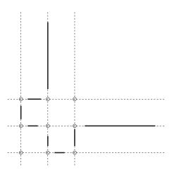
Fig. 5. An overhead view of a floor plan of the scene indicating the walls, which are considered to have infinite extent and are depicted by dashed lines, and the wall segments, which are depicted by the solid line segments. These wall segments correspond to contiguous planar regions in the RGB-D image. The interpretation system also considers all of the possible intersections between perpendicular walls, denoted by circles in the figure, since these may correspond to corners in the scene.
