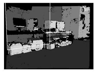
Fig. 7. For each pixel in the frame we can compute the index of the wall that best explains the observed disparity and orientation. We can then evaluate how well a particular wall explains a given image interval by projecting the wall into the frame at that interval and determining how many pixels in that region agree with the proposed label. The quadrilateral demarcated on the frame corresponds to the projection of one of the prospective walls into one of the image intervals.
