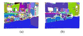
Fig. 4. a. Extracted Planes b. Result after coplanar segments are merged
