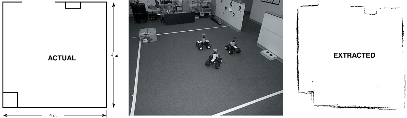
Fig. 10. Cooperative mapping with three robots, in an environment with real and simulated walls.
