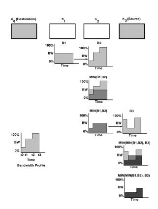
Figure 3. Calculating a bandwidth profile.
