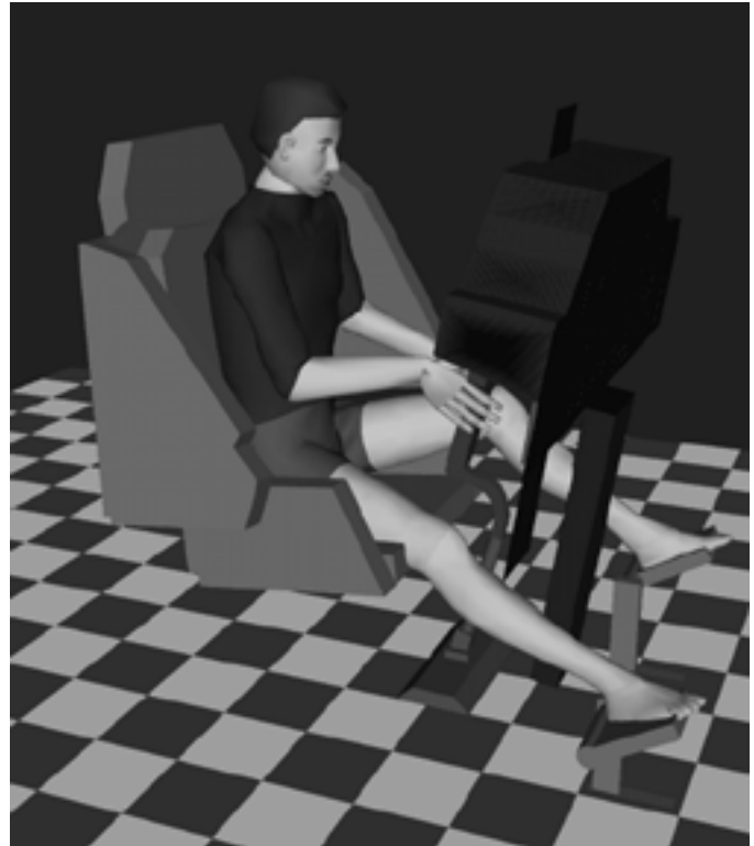
Figure 2. Smooth body Jack as virtual occupant in an Apache helicopter CAD model.
